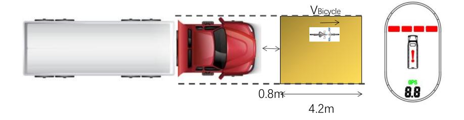
V<sub>VRU</sub>: Target object speed
